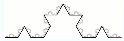
Figure 9.11. Measuring the length of the Koch curve with step sizes of 1/3^m . Here m = 2 , so the step size is s = 1/3^2 = 1/9 . The number of steps is N = 4^2 = 16 , and the estimated length at this stage is N \cdot s = 16/9 .
